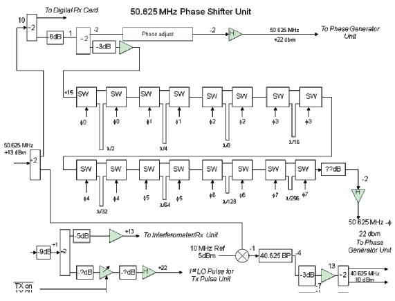
The RX summing unit is then transferred the signal with Doppler frequency from  $f_{TX} + (0 \text{ to } 15\Phi)$  to  $f_{IF}(40.625 \text{MHz}) + (0 \text{ to } 15\Phi)$ , based on which the signal is digitized and Doppler frequency is then picked up.
